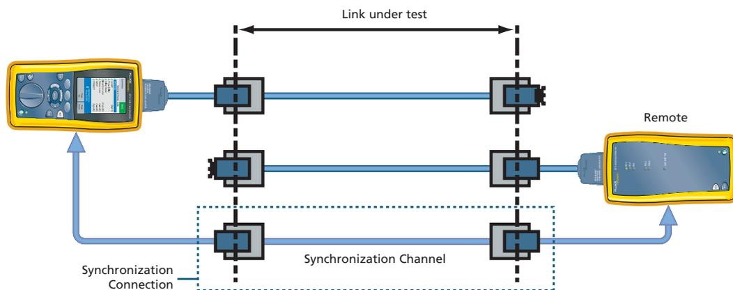
Figure 5 – Pair-to-pair Alien FEXT measurements. The main and remote units are plugged into different cabling links at opposite ends of bundle under test. A spare channel in this bundle connects the synchronization modules plugged into each of the testers to allow the testers to perform all of the pair-to-pair FEXT measurements between the wire pairs of two selected cabling links.
