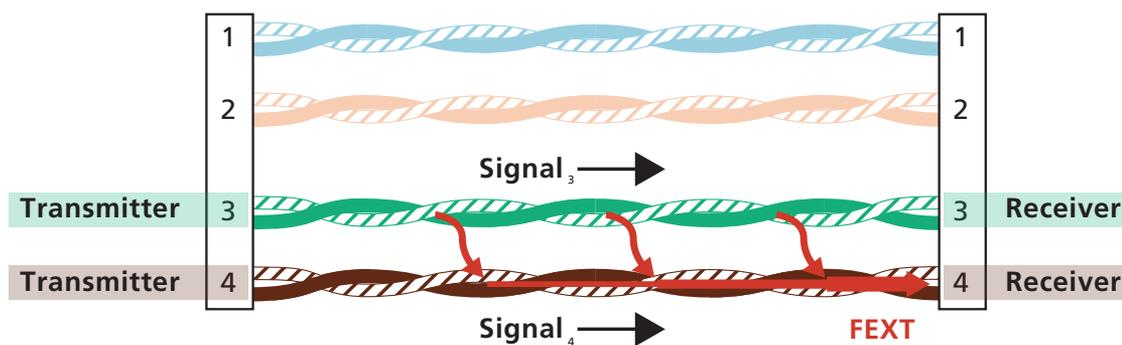
Figure 2 – Far-End Crosstalk (FEXT) measures the crosstalk induced in wire-pair 4 that travels the length of the cable in the direction of the transmitted signal and competes with the clarity of “Signal 4” arriving at Receiver 4.
